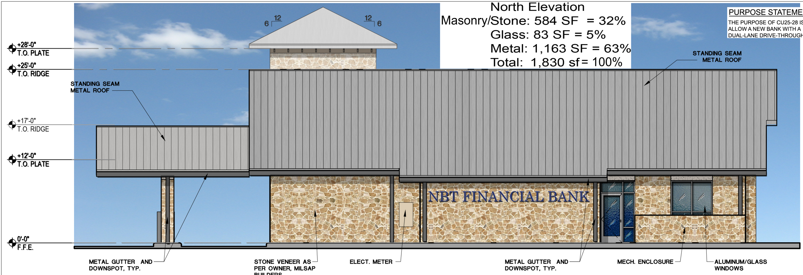
NORTH ELEVATION SCALE: 1 : 50
